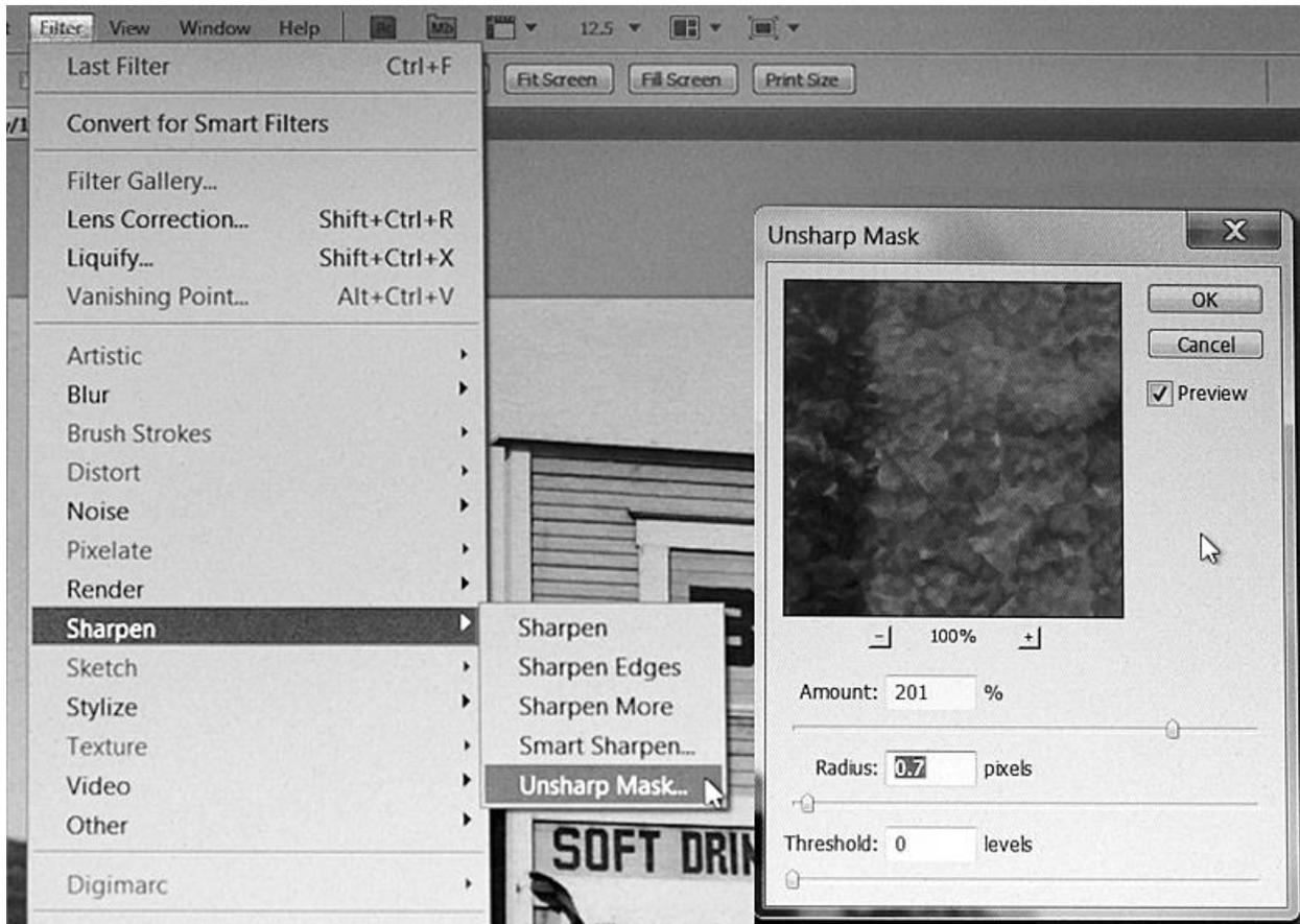
I recommend at least the initial sharpening use a radius of 1 pixel or less. I have the image at 100% to judge how much is needed. Usually, I'll sharpen incrementally and selectively, using the duplicate layer and eraser method. Also, to avoid over sharpening I like to have the image at 100% magnification. Sometimes I'll apply sharpening just to critical edges and, on faces, just to eyes, and sometimes teeth and lips.
